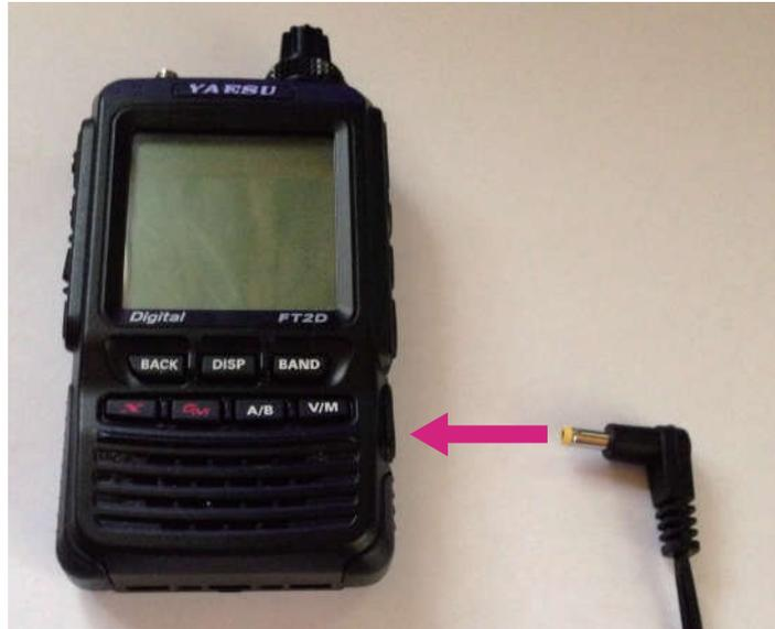
3. Press and hold
