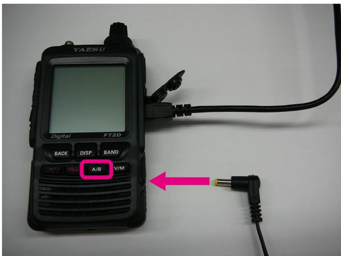
The power turns ON and you will hear a “beep-boop-bop” sound. On the FT2DR/DE display, “---DSP WRITE MODE---” and “Push DISP Key!” will appear.
