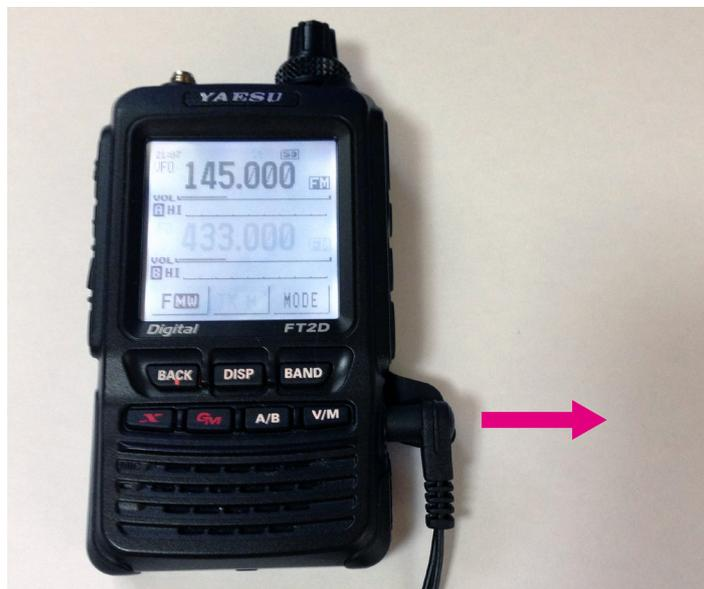
5. Use the supplied cable to connect the FT2DR/DE DATA terminal to the computer.
