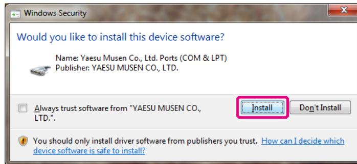
The device driver installation begins. When the installation completes, the message "Windows has successfully updated your driver software" will appear.
