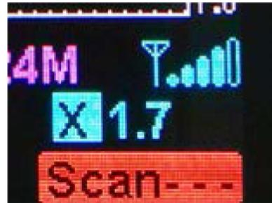
4, on the Single scanning screen, there is a S-Antenna signal strength indicator, which is a rough indicator of the antenna RF field.
