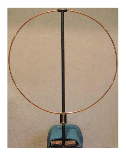
You may paint the antenna but oxidised copper does not affect the operation of the antenna
