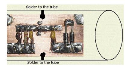
Solder both sides of the PCB to the («fig) inner side of the tube. Start with soldering thick wires to the tube and then solder pcb to the wires.
