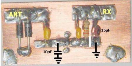
The INA 02186 has a high gain and a good connection to ground is essential. Some home brewers had to deal with an oscillating amplifier. To prevent instability ensure that both lips have direct contact with each other via one track. Do not separated by a machined groove, but solder on the same "island" or track.
