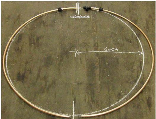
The 15 mm diameter soft copper tubing (from a hardware store) is 4 meters long, actually there are two easy to bend pieces of 2 meters.
