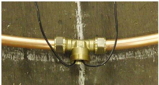
The flexible insulated wire does not need to be concentric.
