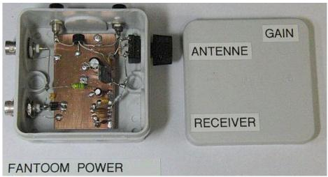
In previous schematic 330 ohm resistor was 240 ohm. Sometimes the IC was oscillating with short coaxial cable, therefore the resistance was increased and IC's supply voltage was reduced to 5.5 volts.
