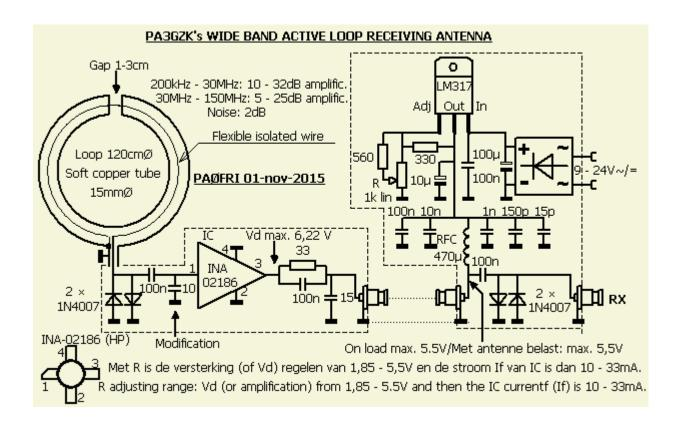
If one has no place for an antenna of sufficient length for receiving radio signals, a small active antenna may be the solution and you may find on the Internet a lot of related publications. If you want a system that is able to reduce or suppress interfering signals, most articles are not appropriate! The following design has that noise cancelling quality, you can confirm it by listen to MP3 files later in this article!
