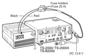
First, connect the DC power cable to the regulated DC power supply; the red lead to the positive terminal and the black lead to the negative terminal. Next, connect the DC power cable to the transceiver's DC power connector. Press the connectors firmly together until the locking tab clicks.
