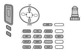
Each time you press the desired key, the Commander will automatically enter transmit mode and send the corresponding control command to the TS-2000 (Transporter).
