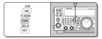
2 Turn the MULTI/ CH control counterclockwise to reduce the power or clockwise to increase the power.
