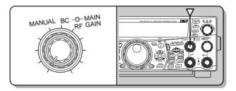
Depending on the type and gain of your antenna, and the condition of the band, you may also prefer leaving the MAIN RF GAIN control turned counterclockwise by the same amount rather than turning it fully clockwise. When using FM mode, always set the MAIN RF GAIN control fully clockwise.
