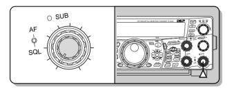
**Note:** The position of the **SUB AF** control does not affect the volume of beeps caused by pressing buttons. The audio level for Packet operation is also independent of the **SUB AF** control setting.
