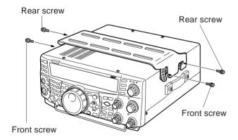
To remove the transceiver from the bracket, first remove the front screws, then loosen the rear screws slightly and pull the transceiver forward to unlatch it from the bracket.
